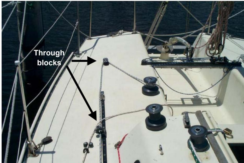
Make sure the forward (clew) end of the genoa sheet is routed outside the shrouds and up to the bow. Position the block on the track to the appropriate position (marked on the deck) for the sail we will have up. Route the jib sheet UNDER the twing line. Route the end through the bottom of the back block and around the winch. Make sure the winch handles are out and in their pockets.
