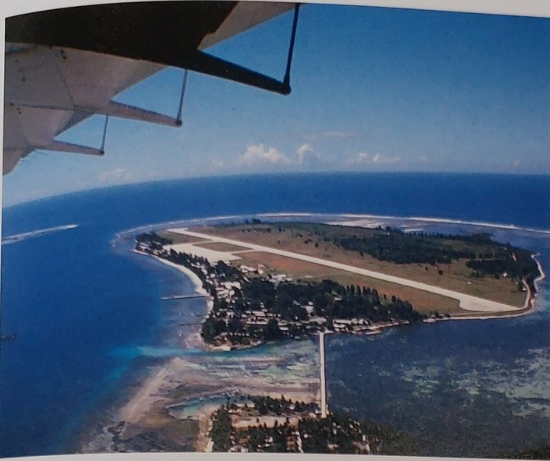
The runway on Gan Island was first constructed of steel sheeting in 1941. It was later upgraded by the British in 1957. At its peak in 1960 – 61, it handled 12,500 passengers.
