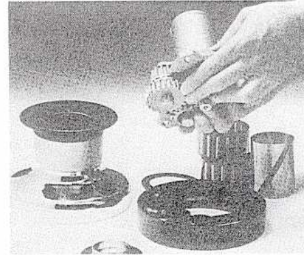
8 (a) Re-assemble parts into pedestal with clutches marked "C" on central shaft for clockwise rotation. For anti-clockwise rotation, assemble clutches marked "A" on to central shaft.
