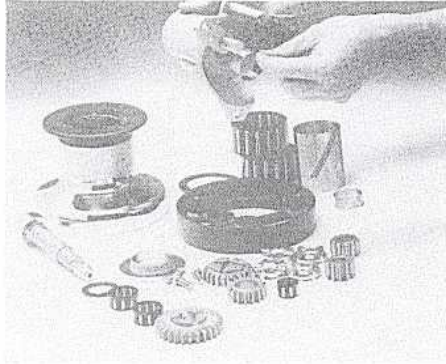
5 (a) Remove all parts by hand including drive shaft, bearings and stainless steel bearing races from inside top and bottom of pedestal (Models 22 through 29 only).
