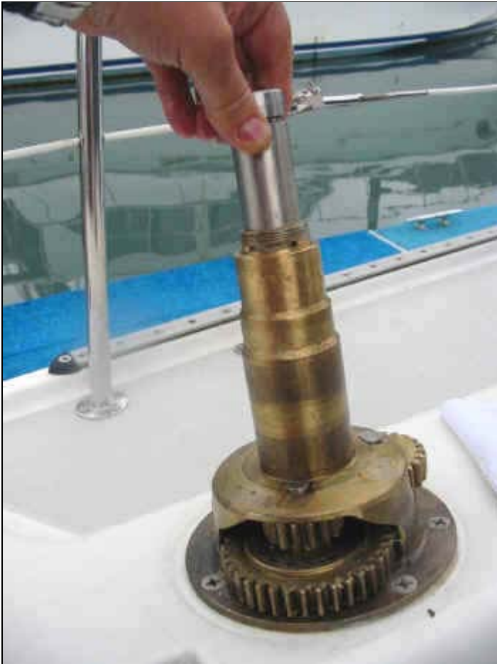
Place the main spindle back in the center stem (with the geared side down).
