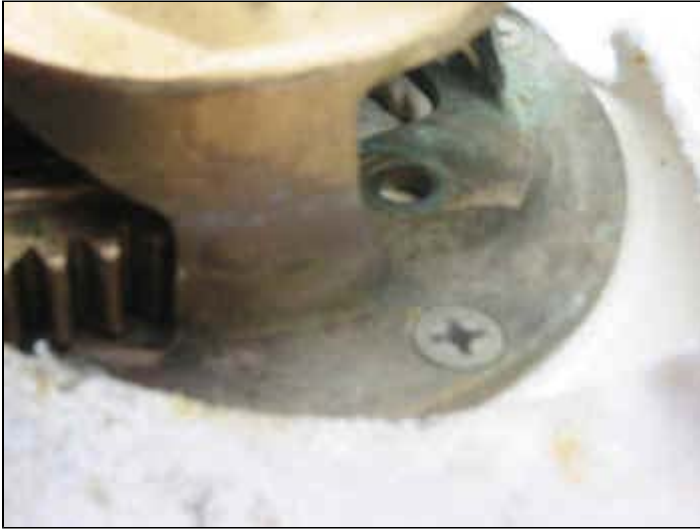
Check the bottom of the Center Spindle for dirt/crud.
