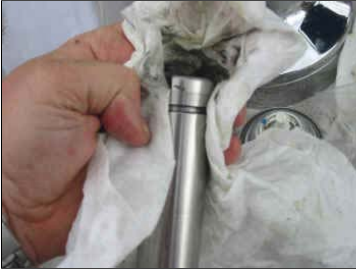
Clean and lubricate the main spindle.
