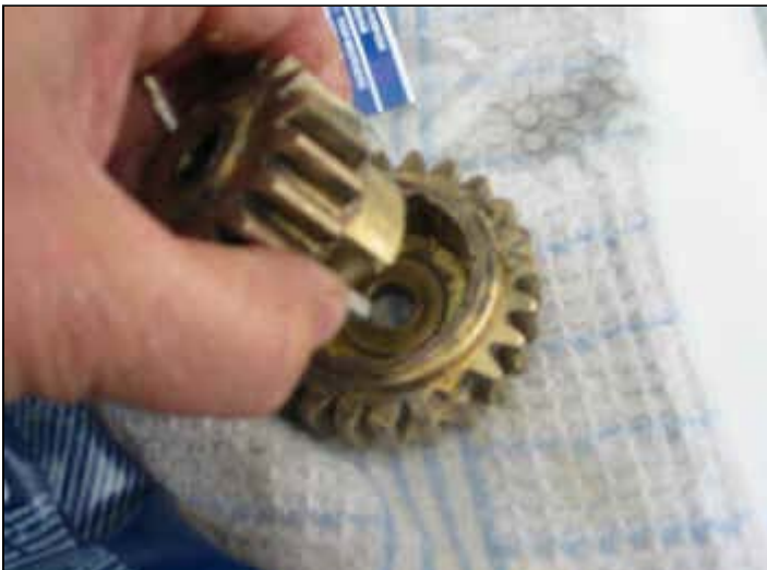
And reassemble it by pressing in the pawls
