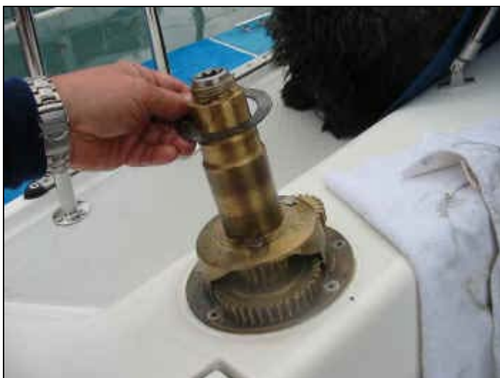
and place it over the center stem, pressing it down as far as it will go.
