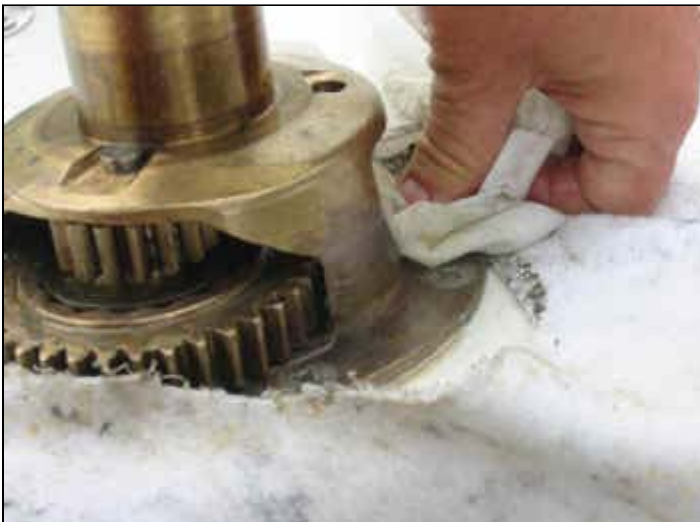
Clean out the other side of the housing for the gear assembly,
