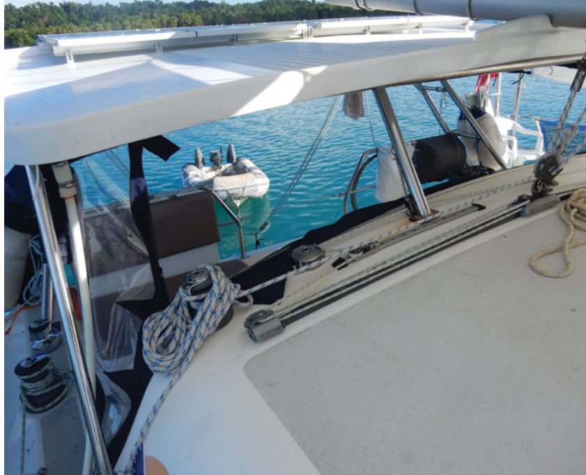
Rain-catching hardtop with solar panels and boom crutch.
