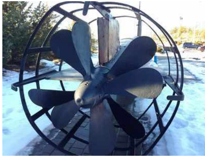
Counter-Rotating Propellers on Japanese Mini-Sub HA-8 in the Submarine Force Museum in Groton, Connecticut
