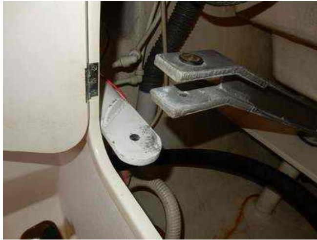
Disconnecting the Rudder Arm Prior to Dropping the Rudder
