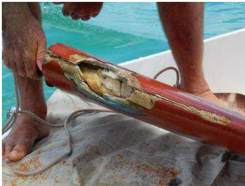
The Leading Edge of the Rudder with Exposed Interior Filler
