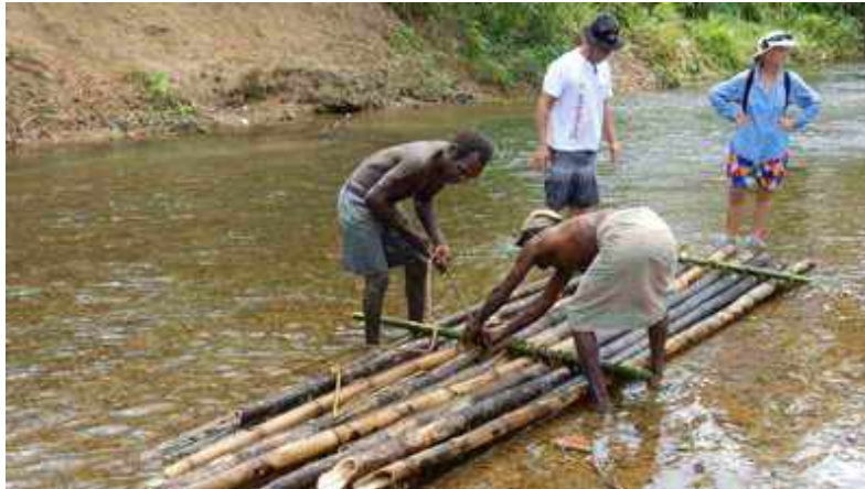
Bamboo logs being tied together with strong pliable vines.
