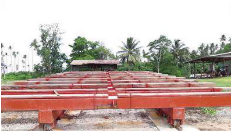
The 200 ton trolley- about 24' wide but extendable
