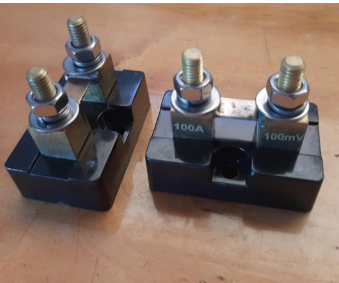
Reidon shunts 100mv, 200a
