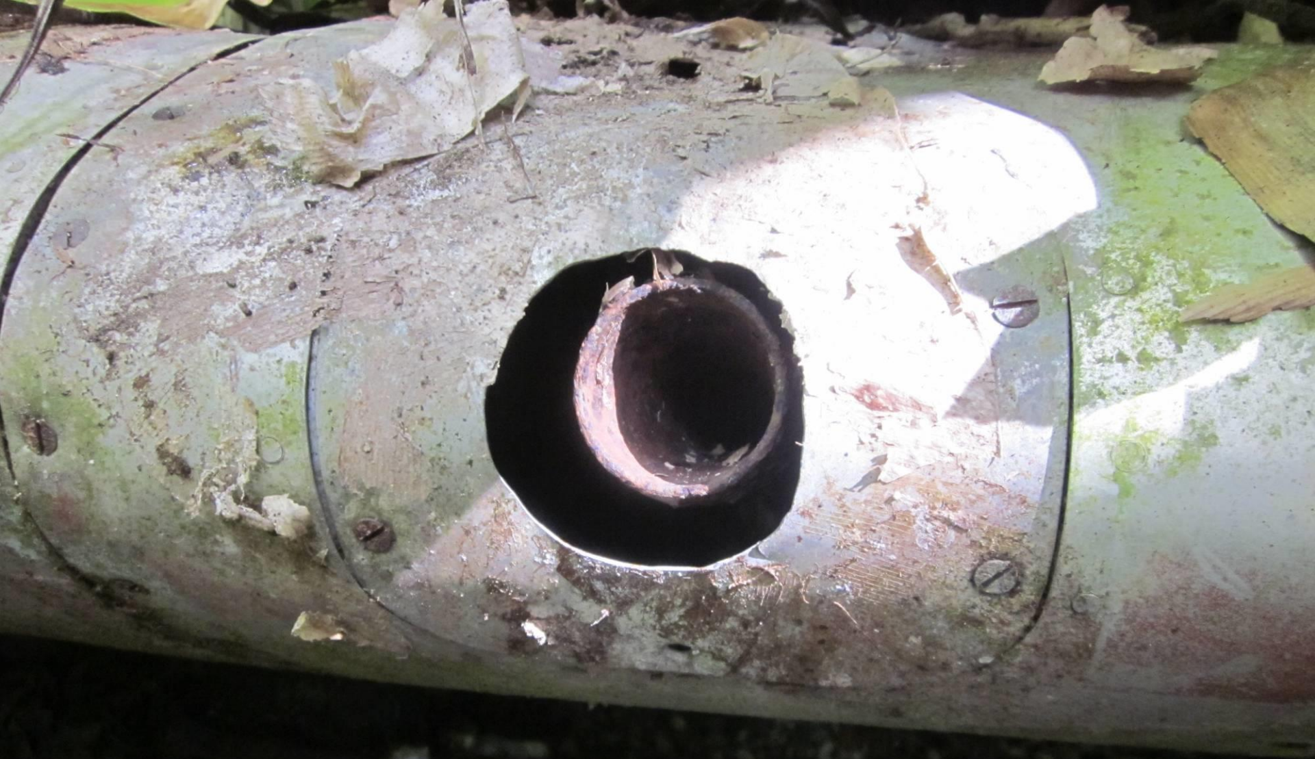
A6M Zero 20mm wing cannon
