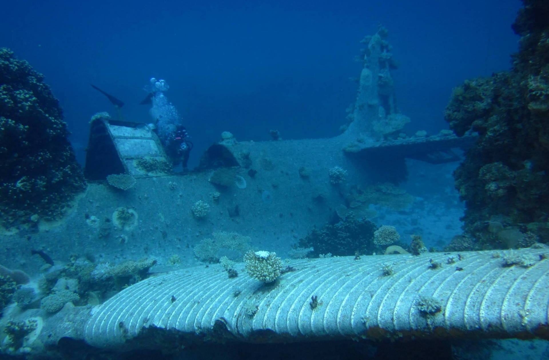
Unique TBD wing surface ridges, Sherry inspecting bomber and gunner's seats
